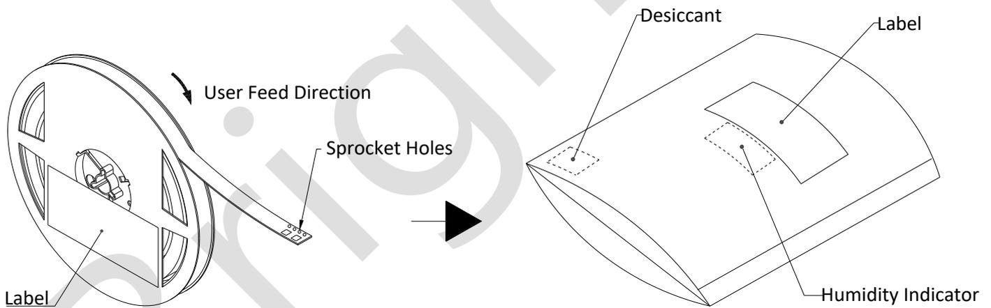
1. Moisture-sensitive product is packed in a dry bag containing desiccant and a humidity card according JEDEC-STD-033.
