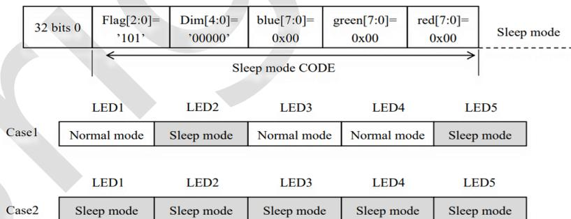
In Case 1, if LED 2 is in sleep mode, during the subsequent data transfer process, the state of LED 2 will remain unchanged as long as 32 bits of data for LED 2 is received with Flag[2:0], DIMMING[4:0] set as 8h"A0". This indicates that LED 2 will remain in sleep mode. In this scenario, LED 2 can relay the remaining 32 bits of data to LED 3 to modify the display data of LED 3. In essence, the inactive chip (LED 2 in sleep mode) has the capability to relay data to the subsequent chips.
